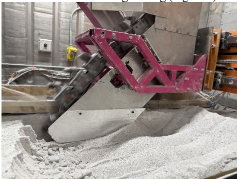
Figure 1: Icy regolith simulant excavation with chain trencher.
